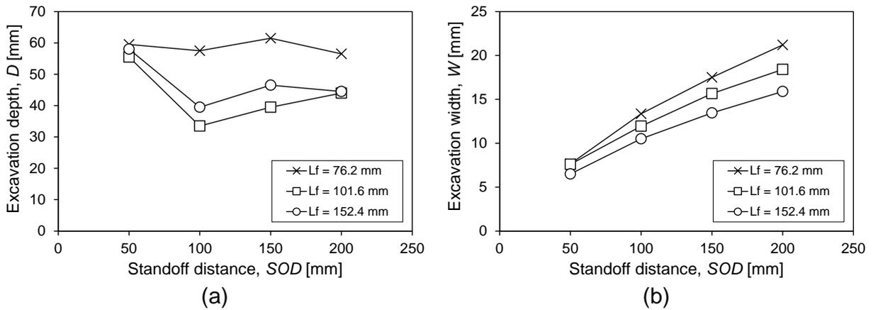
Fig. 3 Rock excavation performance of abrasive waterjet: (a) excavation depth and (b) excavation width with abrasive flow rate of 5.6 g/s
