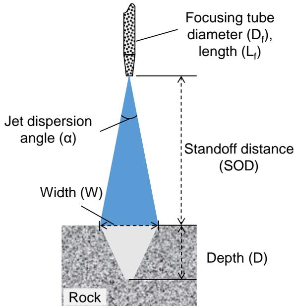
Fig. 2 Concept of jet dispersion for underground excavation with abrasive waterjet
