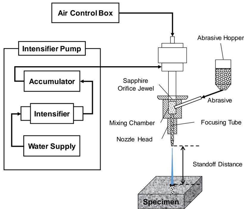
Fig. 1 Schematic of abrasive waterjet system (Hwang et al. 2019)
