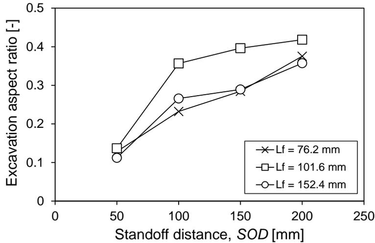
Fig. 4 Effect of standoff distance and focusing tube length on the excavation aspect ratio
